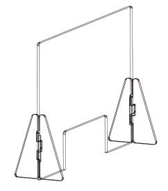
"Cachiiina horizontal type" is an acrylic partition. All parts are made of acrylic. No metal parts are used. No adhesive is used for assembly, so you can freely disassemble and assemble
